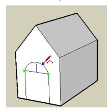
6. Use the **Eraser** tool to erase the top edge of the rectangle, so the door is one face.
