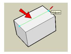
3. Use **Move** on this line, pulling it up (in the blue direction) to make the roof.
